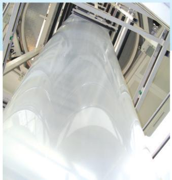
layers, is one of the most precious factors of the significant experience acquired by COLINES® in the blown technology. The minimum thickness of the film produced is of 24 micron with sigma ± 0,7, with a central barrier layer of 3 micron of EVOH, suitable for food packaging as well as medical applications. The net hourly throughput is of 400 kg/h. ==v/bs
