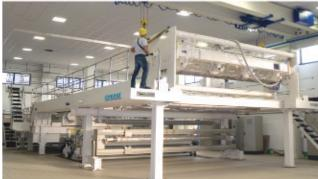
top: cast line for CPP film, web width 4500 mm. In assembling bottom: view of the green area around Colines® Azzate factory
