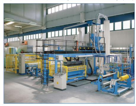
Among the noteworthy features of this line, it is worth mentioning the **automatic** turret winder with two axes, roller unit and in-line cutting, and the edge trim suction system for in-line recovery, equipped with a **video inspection** system. Colines® is the leading manufacturer of extrusion lines to produce air bubble film. With more than 200 lines sold all over the world and more than 35 years of experience in this field we can guarantee quality, performance, assistance and reliability.
