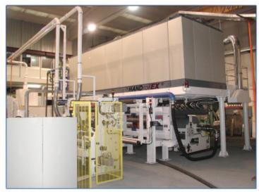
The winding system, moreover, allows an even larger functionality, since with the same structure it is possible to use 2" and 3" cores, for a 2000 mm wide line is possible to place no.2 1000 mm winding modules side by side, and in addition to **modernize** already existing lines with this innovative winding units. 16007
